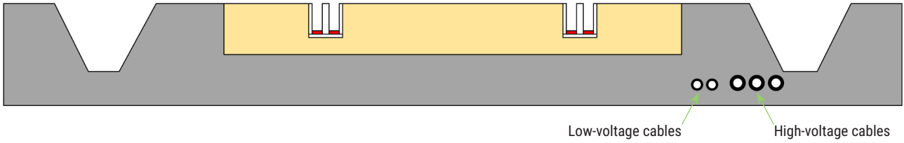
Figure 5: Cross-section of a road equipped with Elways double rail. These rails are powered from low-voltage cables that ensure rapid switching between segments. The low-voltage cables are themselves powered from the high-voltage cable. Source: Elways.
