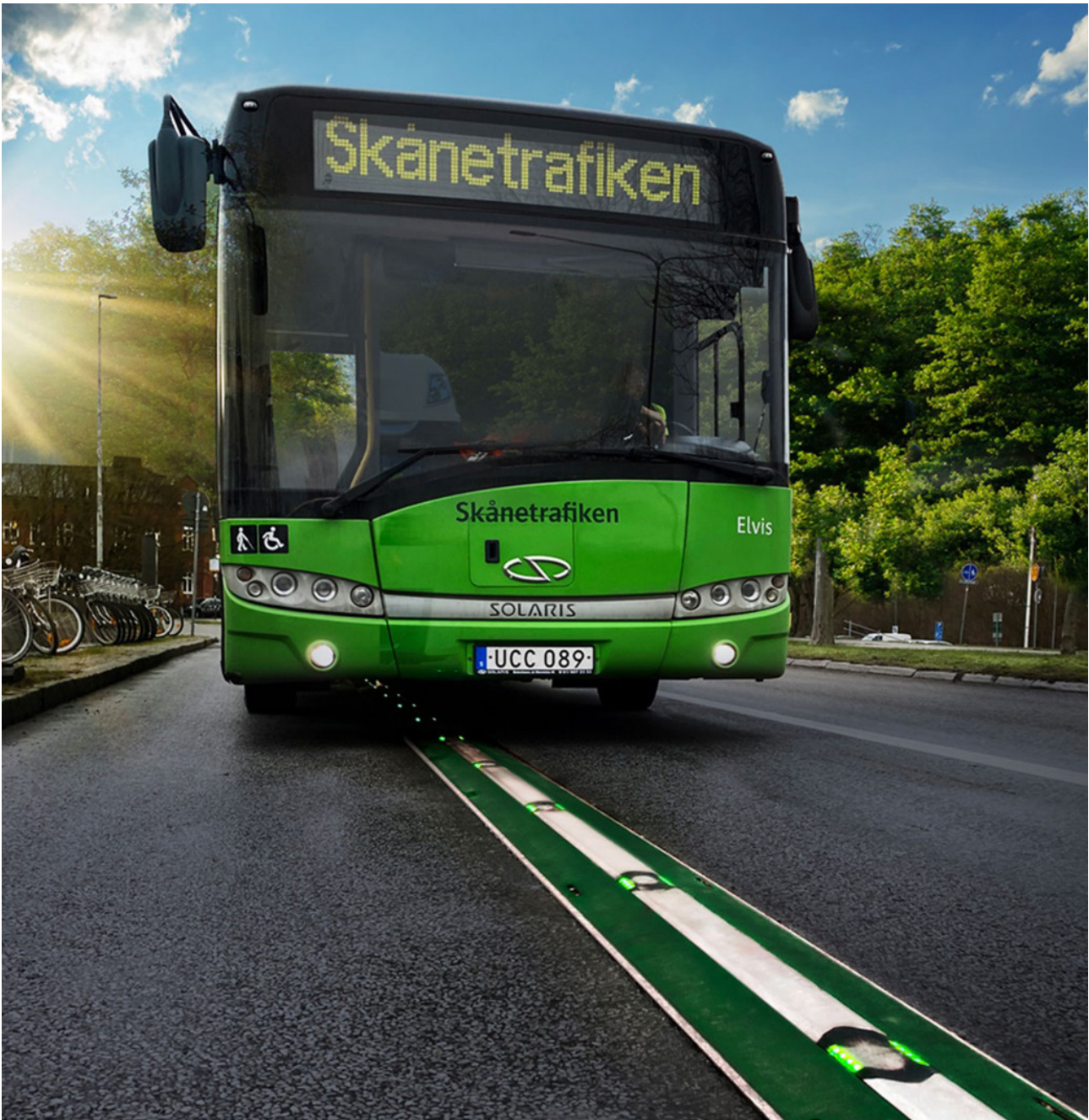
Photo 5: A 1 km trial of the Elonroad solution in Lund (Sweden).
