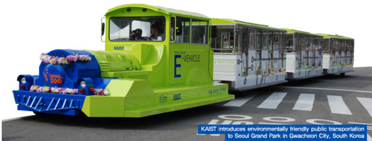
Figure 7: Tourist train charged by induction while running in a park in Seoul – KAIST.
